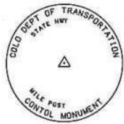
Typical Control Monument Cap Not to Scale
