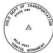
Typical Control Monument Cap Not to Scale
