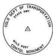
Typical Control Monument Cap Not to Scale
